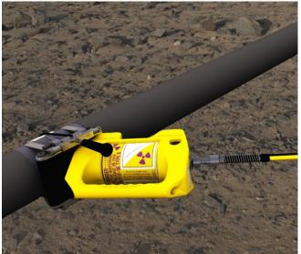
The PipeLiner can be positioned and locked in place at any angle around the pipe.
