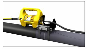
Attaching The PipeLiner accessory converts the Sentinel<sup>™</sup> 880 series projectors into dual purpose exposure devices for pipeline radiography.
