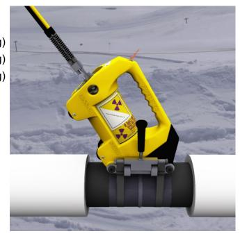
The PipeLiner is clamped with a polymer coated webbing rated to 1000 pounds breaking force, with an operating range of +  $75^{\circ}$  to -  $60 \text{ C}^{\circ}$ .
