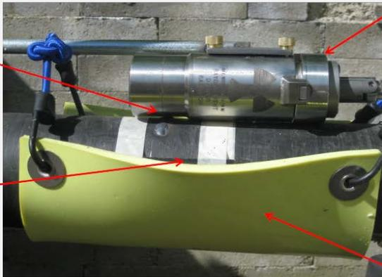
SCAR device in contact with pipe
