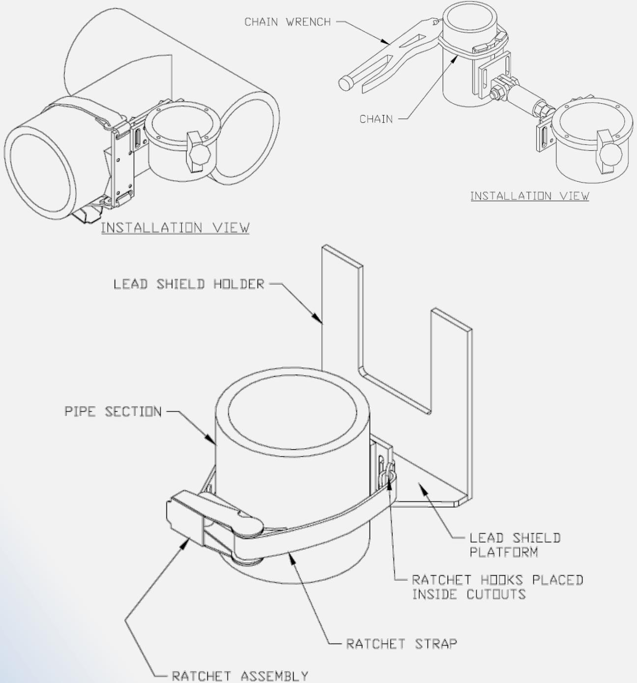
FIGURE 4 - SHIELD HOLDER INSTALLATION
