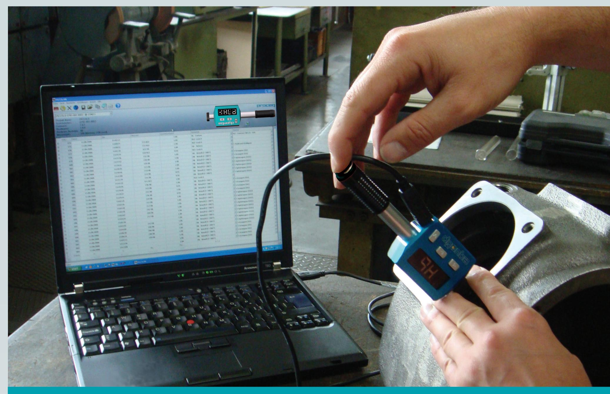
Portable Metal Hardness Testing
