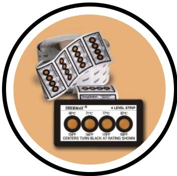
Simply remove the adhesive backing, and press label firmly onto a clean dry surface. When the rated temperature is reached, the dot(s) in the middle will change and remain black indicating that the desired temperature has been reached.
