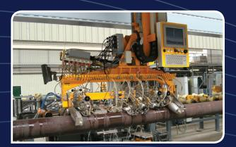
The inspection of the weld is performed by several sets of wedged linear PA probes by electronically steering an array of angled UT beams.
