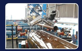
A variety of ultrasonic configurations according to inspection requirements and site conditions are available. Both static and moving inspection head configurations are available to accommodate different site conditions and throughput requirements.
