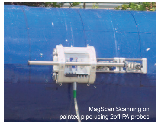
MagScan configured for Girth Weld Inspection (2 ToFD and 2 P/Array Probes)
