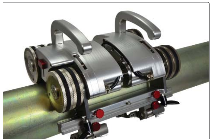
Circumferential Scan, With Handles
