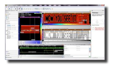
Full recordability of data when using the Prisma is standard, which means that screenshots and all data can be retained and analyzed at a later date using UT Studio. IN using the full data gathering capability - traceability can be achieved; hence repeatability of the inspection and results can be confirmed.
