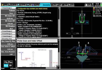
In stop mode the veo system is able to display four screens of information simultaneously. For example a Configurations Summary, Help Page, Plan view of Inspection (showing expected probe movement), 3D Scanplan (showing the probes, parts, inspection beams and planes of focus - as above). Any one of these can be maximised to a full screen view.
