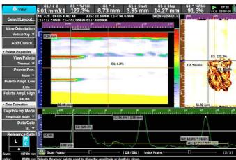
The VEO offers full merged C-Scan capabilities allowing the inspector to see the complete area of inspection. TOP views (from angled or normal beam inspections) or C-Scans (from normal beam inspection) can be produced based on either amplitude or time of flight data. C-Scans from multiple passes can be merged together.
