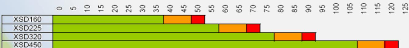
Recommended Steel thicknesses per XSD - SFD700 - OptD 2 - Film ISO 320 - Simple film
